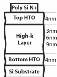
Fig. 1: Schematic showing the capacitor device stack studied in this work. Various high-k were investigated: \text{HfO}_2 , \text{Al}_2\text{O}_3 and HfAlO with different Hf:Al ratios (9:1, 1:4 and 1:9).
